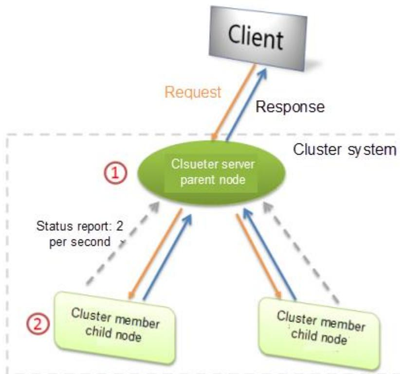
Fig. 2 Cluster communication mechanism
